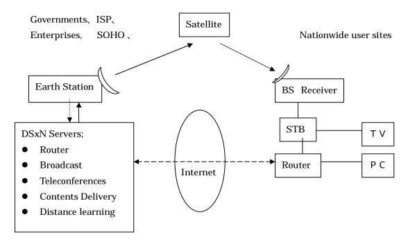
System Configuration of Direct Satellite Inter-Net
